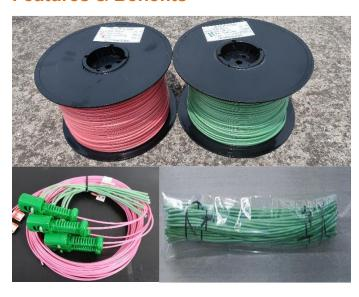
*HiCORD*<sup>®</sup> consists of polypropylene code with a variety of colors, a bobbin made by forfeited compact paper, and PETN as the ignition explosives.
